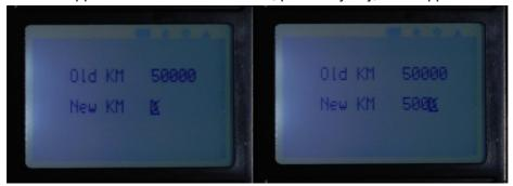
Note: Some instruments, need to manually enter the old mileage, and some instruments can be directly read the mileage. If the mileage can not automatically read the meter, enter the current mileage meter, for example, the A6L Marelli instrument which is CAN interface, need to manually enter the old mileage.
