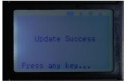
Note: After Odometer adjustment is successful, device will automatically reset instruments. After that, some instruments need to disconnect the fuse, and then re-power. Set correct date and time before we can work, for example: the audi a4 RB4, RB8 instruments, if not do that, it will appear the symptoms, can't ignition.
