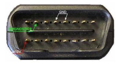
Apply +12V power supply and push RED or YELLOW button on the Opel Airbag Tool. Opel cars 1997 airbag sensor with yellow or orange 30-pin connector.
