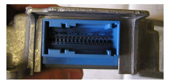
You can connect this sensor on the table and erase crash data using our Opel Airbag Tool.Use this wiring:Airbag sensor: K-line = pin 37 (connected with car OBDII connector pin 12), GND = pin 7, +12V= pin 35, airbag lamp = pin 6; Opel Airbag Reset Tool: K-line = pin 12, GND = pin 4+5, +12V = pin 16
