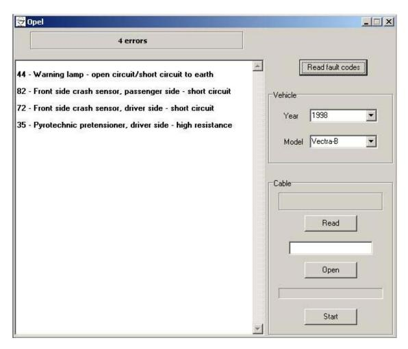
This program works only with Opel Airbag Reset Tool hardware. Connect Opel Airbag ResetTool to car OBDII connector, select car year and type and type read fault codes. Works only with original COM port.
