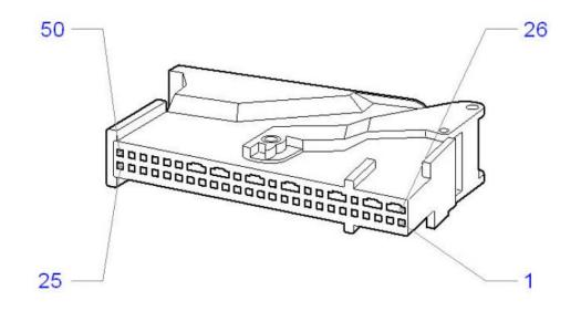
You can connect this sensor on the table and erase crash data using our Opel Airbag Tool. Use this wiring: Airbag sensor: K-line = pin 37 (connected with car OBDII connector pin 12), GND = pin 6, +12V= pin 9, airbag lamp = pin 7; Opel Airbag Reset Tool: K-line = pin 12 or 7, GND = pin 4+5, +12V = pin 16
