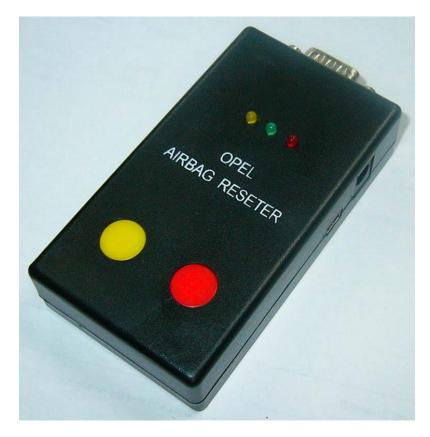
When we apply the +12V power supply to Opel airbag reseter ,the yellow light will flash 10 times,this indicates the system checking .After this we can do the normal operation.
