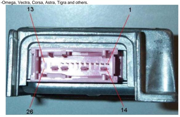
You can connect this sensor on the table and erase crash data using our Opel Airbag Tool. Use this wiring:
