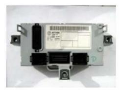
In the immobilizer unit that is seen above, there is an eeprom called 93c66. After this eeprom is read you have to send it to our machine. (Processor must be read as a \*Bin file)
